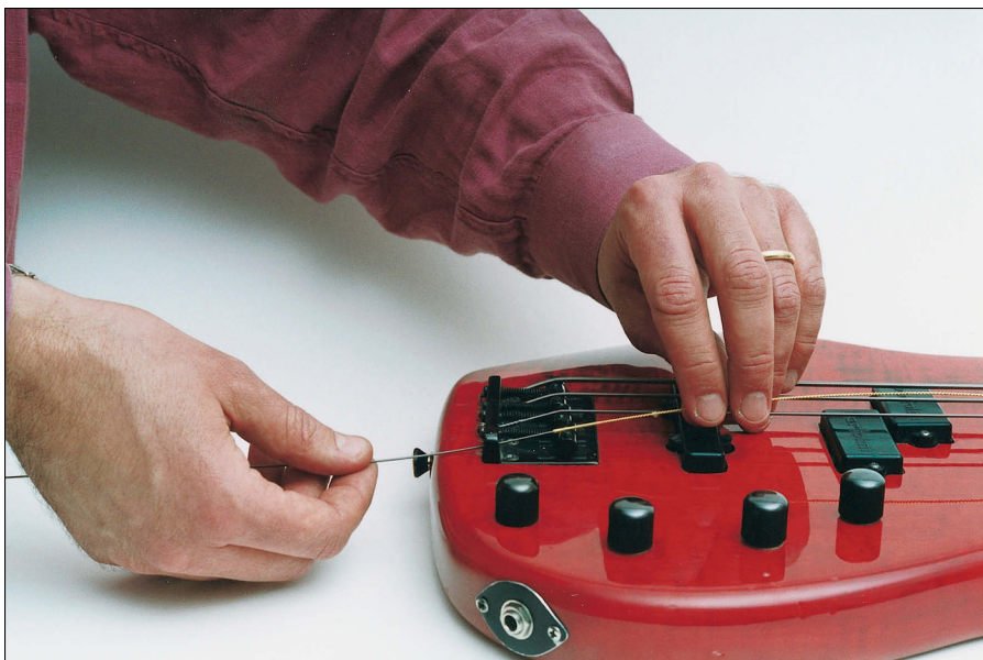
Figure 17-4: Pulling the string through the bridge.
