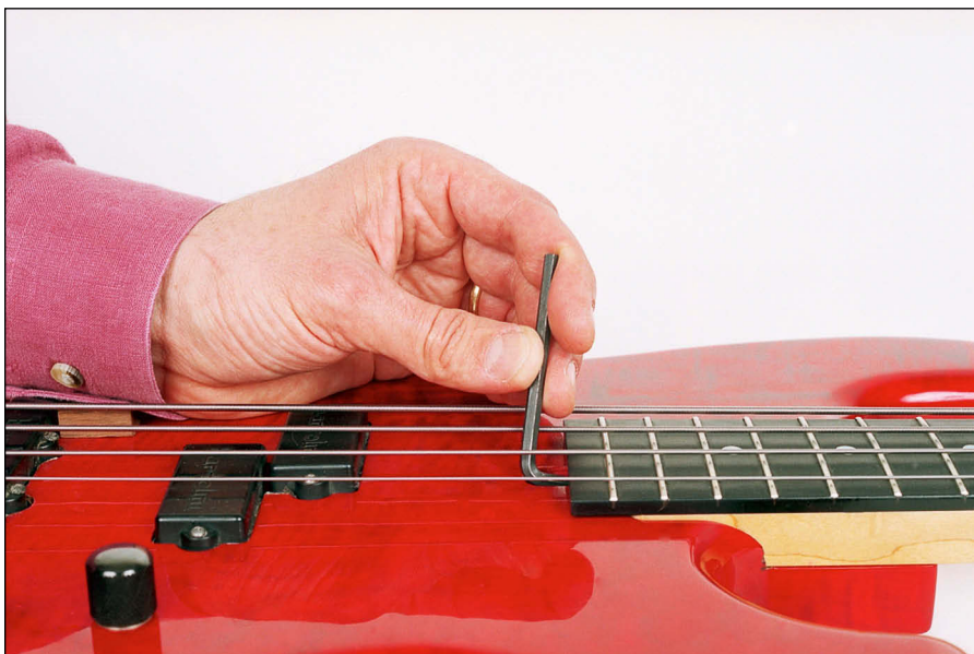
Figure 18-2: Adjusting the truss rod.
