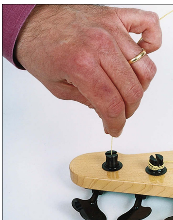
Figure 17-6: Inserting the string into the tuning post.
