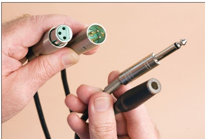
Figure 17-4: 3-pin XLR female and male connectors (left), and a ¼-inch phone plug and jack.
