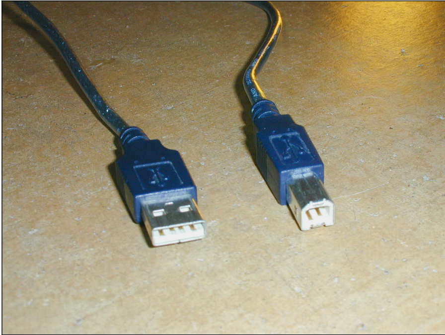
Figure 3-8: USB uses two types of connectors: the “A” connector (left) and the “B” connector (right).
