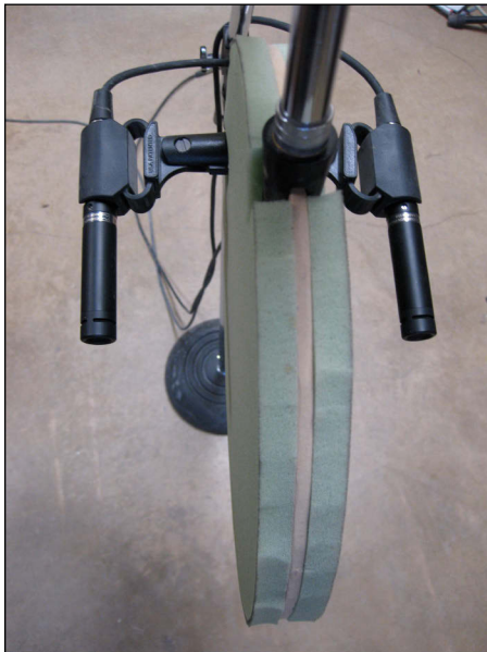
Figure 8-8: A Jecklin disk can make stereo recording easy and capture an awesome, natural sound.
