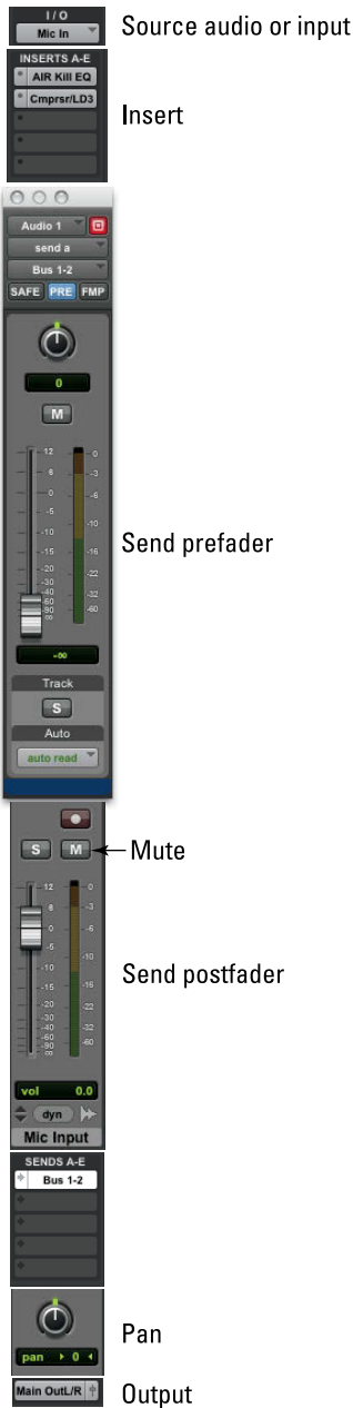
Figure 4-7: Sound travels through the channel strip from top to bottom.
