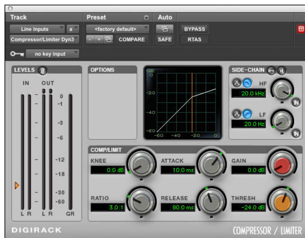
Figure 15-3: Dynamics processors allow you to control the levels of your signals.
