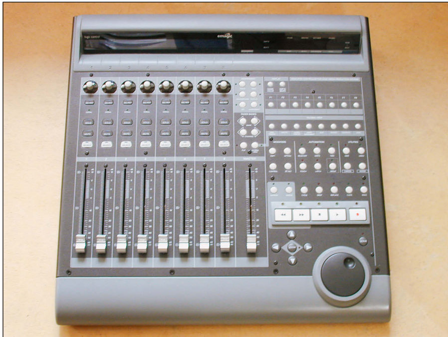
Figure 4-4: A computer control surface acts like a digital mixer for a computer-based system.
