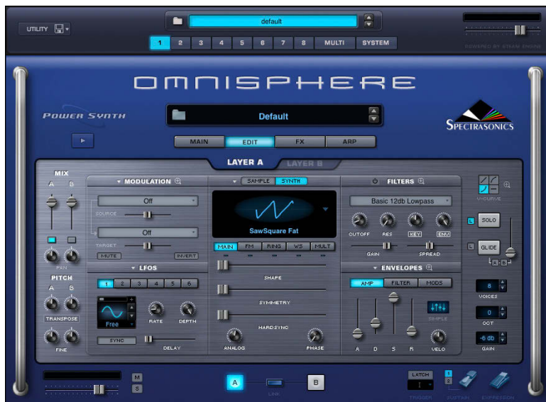
Figure 5-5: Computer-based DAW users can choose soft synths to create their synthesizer sounds.
