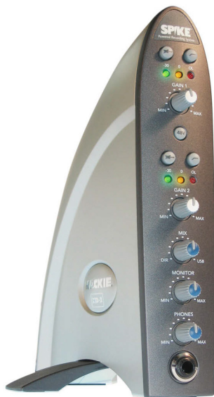
Figure 2-5: A USB interface connects to your com- puter's USB port.
