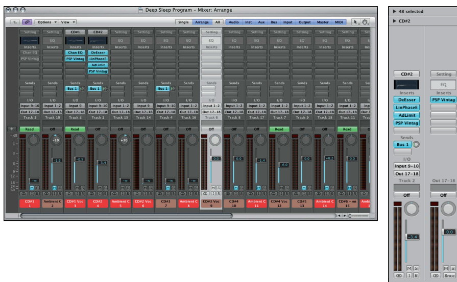
Figure 14-1: The main mixer menu in a software mixer (left) and the channel strip section of the mixer (right).
