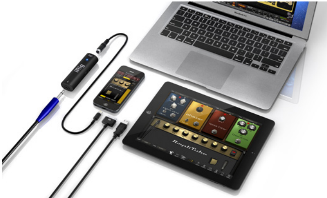
Figure 6-2: IK Multimedia's iRig HD instrument interface offers detachable cables for Lightning, 30-pin, and USB (Mac) connections.
