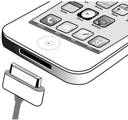
Figure 2-1: The venerable 30-pin connector.
