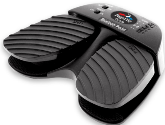
Figure 8-9: The PageFlip Cicada, a Bluetooth page-turning pedal.
