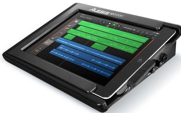
Figure 5-3: The Alesis I/O Dock II is both an audio and a MIDI interface.
