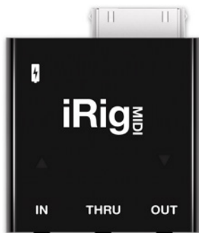
Figure 5-4: The IK Multimedia iRig MIDI 2 is a small MIDI interface that connects to your iOS device's dock port.
