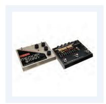
A **delay pedal** allows one or more echoes to be heard after you play a note. A short delay is called a *slapback*. Many early rock and rockabilly records use slapback echoes on guitar and vocals to create a punchy echo. Longer echoes can be used to create intertwining sounds that give the illusion of multiple guitar players. Think of the echo textures of the Police's Andy Summers or U2's the Edge.
